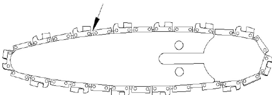
The saw has a screw for adjusting the chain tension. When installing the guide plate, make sure that the adjustment block is in the hole a at the end of the guide plate!
