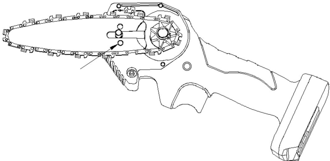
Put the side cover and tighten the screw nut
