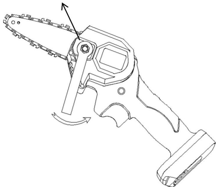
As shown in the picture, twisted the adjusting screw clockwise to tension the chain, counterclockwise is for loosening.
