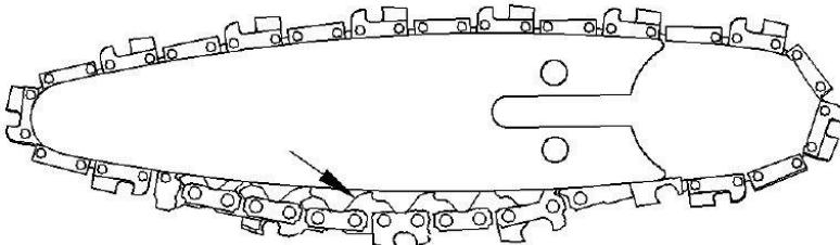
The chain must be stuck to the sprocket. After installation, please check it again.
