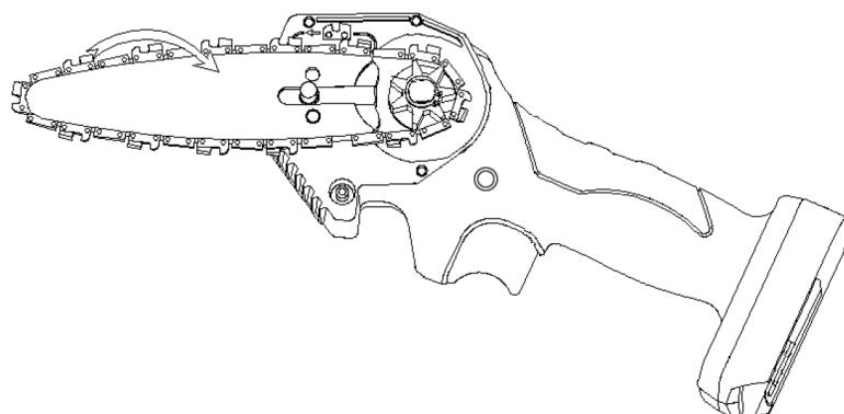
**2.2 How to remove chain?:** After remove the side cover, loosen compression screw, remove the guide and remove chain.
